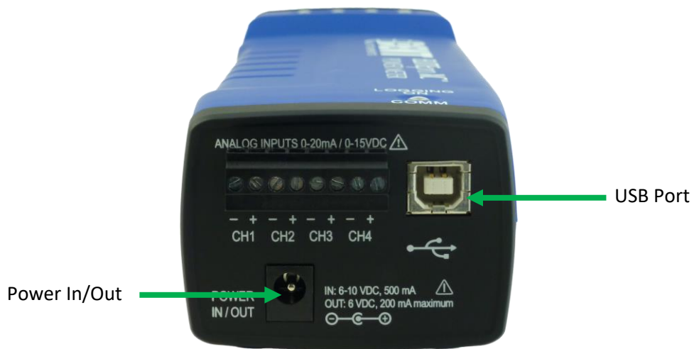
Power End Panel Connections
